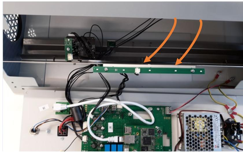
**8.** Unplug particle sensor cable from particle sensor and screw off particle sensor (1x nut)
