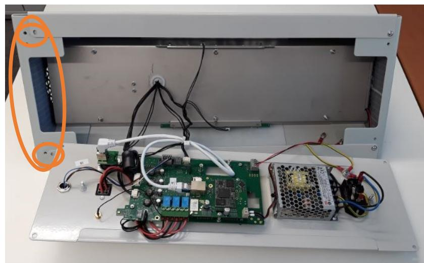
**13.** Place the device lid on main housing, tip it over and connect temperature sensor cable
