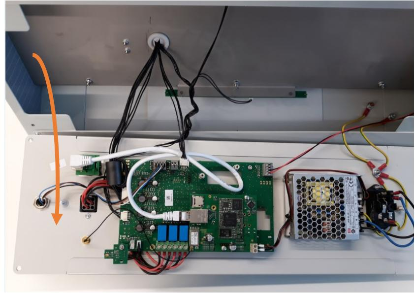
5. Screw off 2 screws and loosen the housing side part
