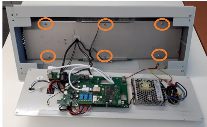
7. Carefully pull off device inner cover forward and place straight into main housing
