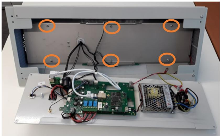
**12.** Slide loosened side part into main housing and screw down (2x screws)
