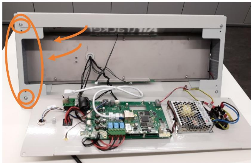
6. Remove device inner cover (6x nuts)
